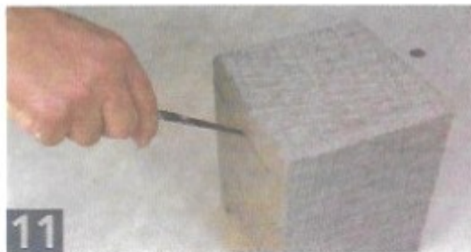
11 Cut the lid off using a knife held at a slight angle.
